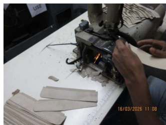
NC- No safety guard in skiving machine.JPG
